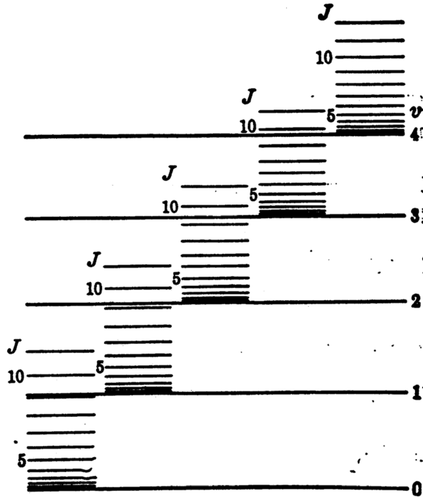
FIG. 53. Energy Levels of the Vibrating Rotator. For each of the first five vibrational levels, a number of rotational levels are drawn (short horizontal lines).
