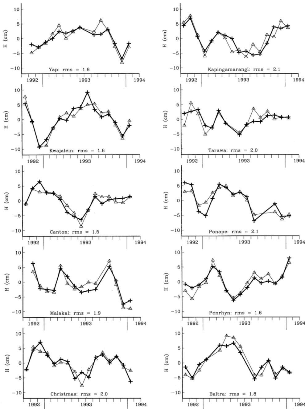
**Figure 5.** Time series from 10 island gauges (thin line) within  $10^\circ$  of the equator at which particularly good agreement was found with T/P data (heavy line). The existence of so many examples such as this argues that T/P is achieving accuracies at the 2-cm level for monthly mean heights in  $4 \times 1$  cells, without orbit adjustment.
